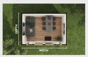
For example, a room with a width of 3.2m (which includes 100mm frame protrusion each side) can't be increased to 3.3m - the next size up would be 3.5m. The maximum width is 5.9m and the maximum depth is 4.4m.
